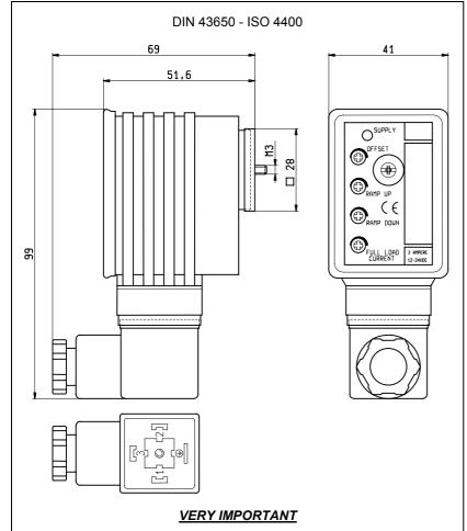
Do not remove the amplifier from the coil while the power is on. This will cause a failure in the internal circuits of the amplifier, resulting in loss of output to the coil.
