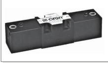
Max. pressure ports P/A/B 320 bar Max. pressure port T 160 bar Max. flow 60 l/min Minimum operating pressure 15 + [0.1 x (pt\*)] bar - see note Maximum operating pressure 250 bar  $10 \div 500 \text{ mm}^2/\text{s}$ Fluid viscosity Fluid temperature 0°C ÷ 75°C Ambient temperature -25°C ÷ 60°C
